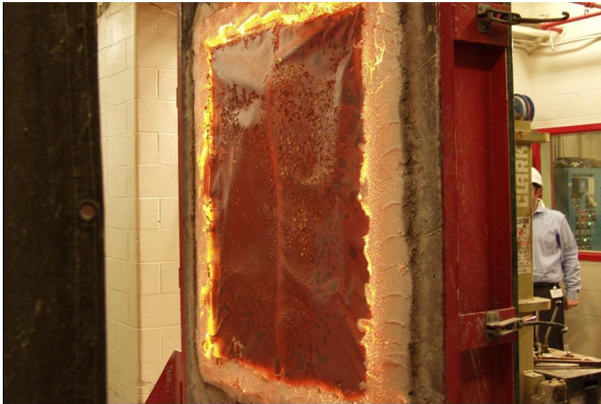
Wall Test – Hot Side
